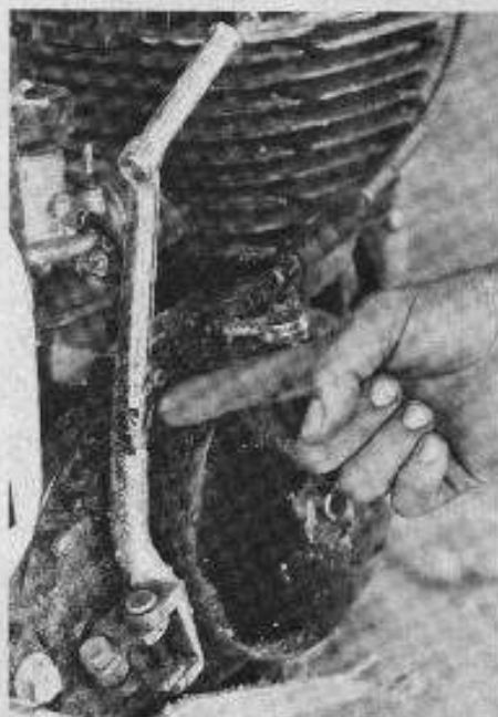
Kickstarter bends out when starting, must be bent in again for riding.
