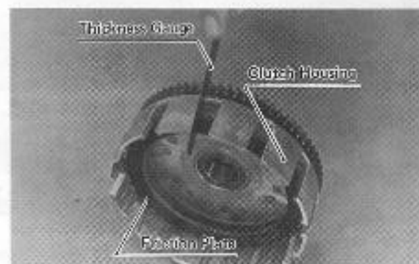
Friction Plate/Clutch Housing Clearance
