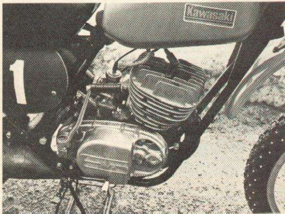
The finning on the cylinder and head of the 250cc engine is different than the production model. The right case cover looks like it once accommodated a carburetor for rotary valve induction. The shift lever has been switched to the right side because that's what Olle is used to.
