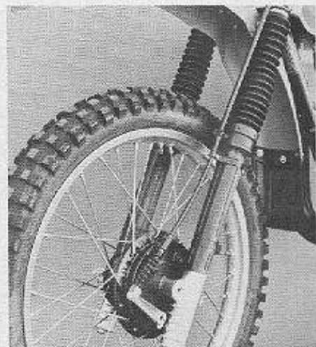
Hollow axle, full-length leg protectors and cast-in cooling fins highlight the 9.25-inch travel front fork.
