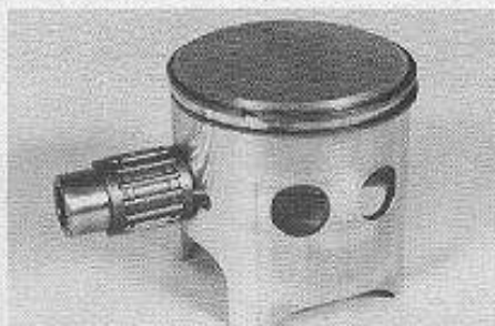
The KX uses a two-ring piston that will require hand-relieving in the contact area with the exhaust bridge.
