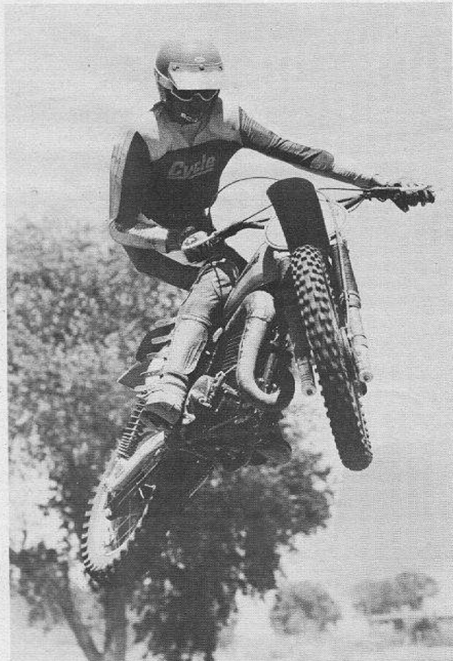
Hollow axle, full-length leg protectors and cast-in cooling fins highlight the 9.25-inch travel front fork.
