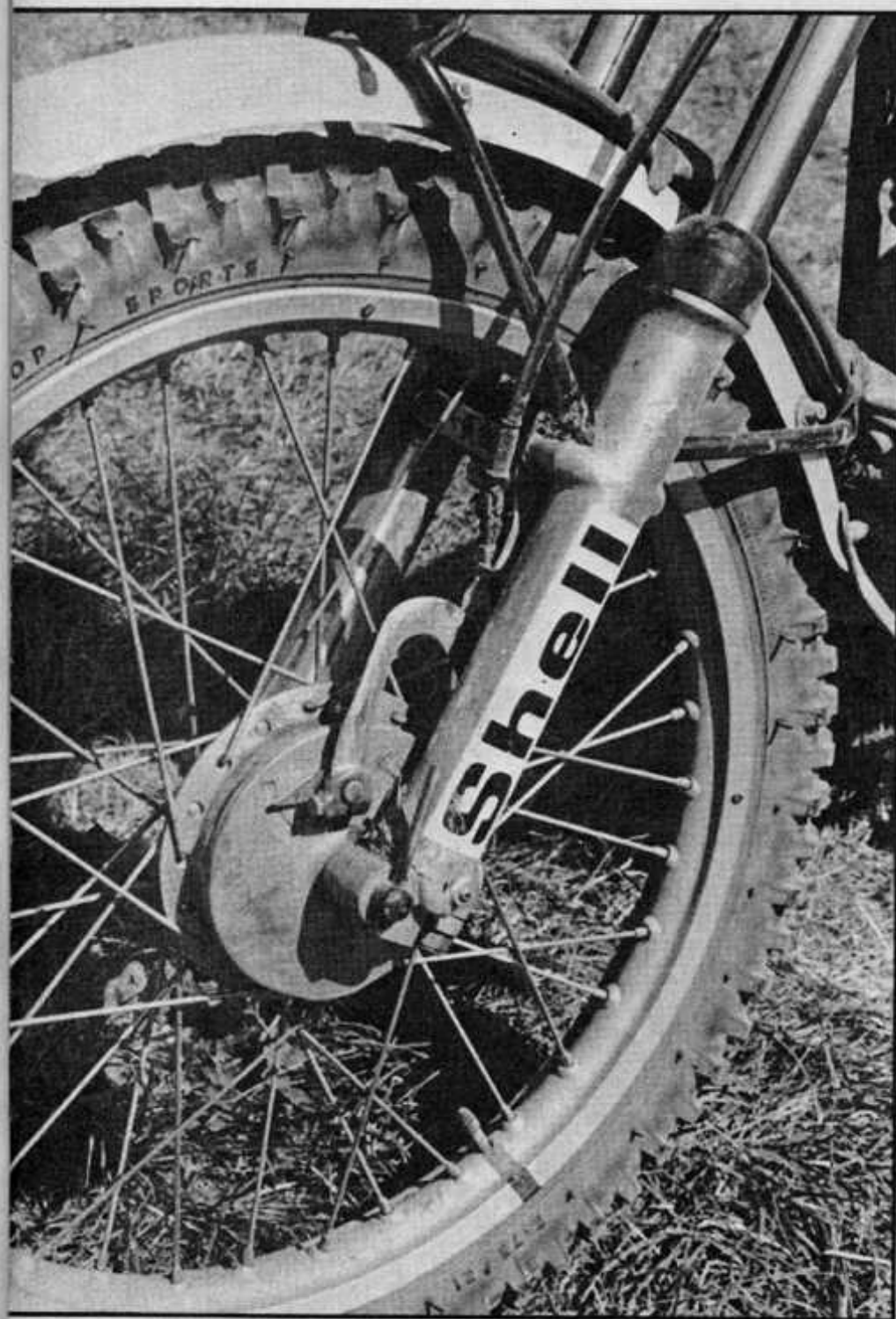
Tucked away brake arm, long travel fork and DID rims.
