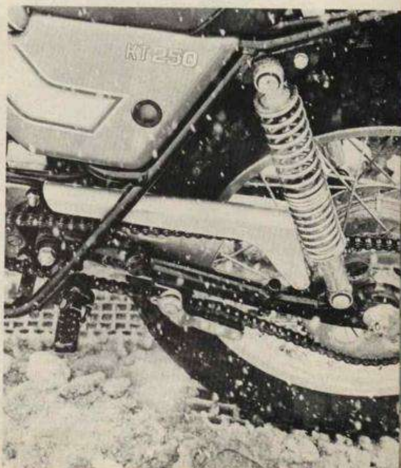
Footpegs, somewhat slippery; chain tensioner, good; shocks, funny looking but functional.
