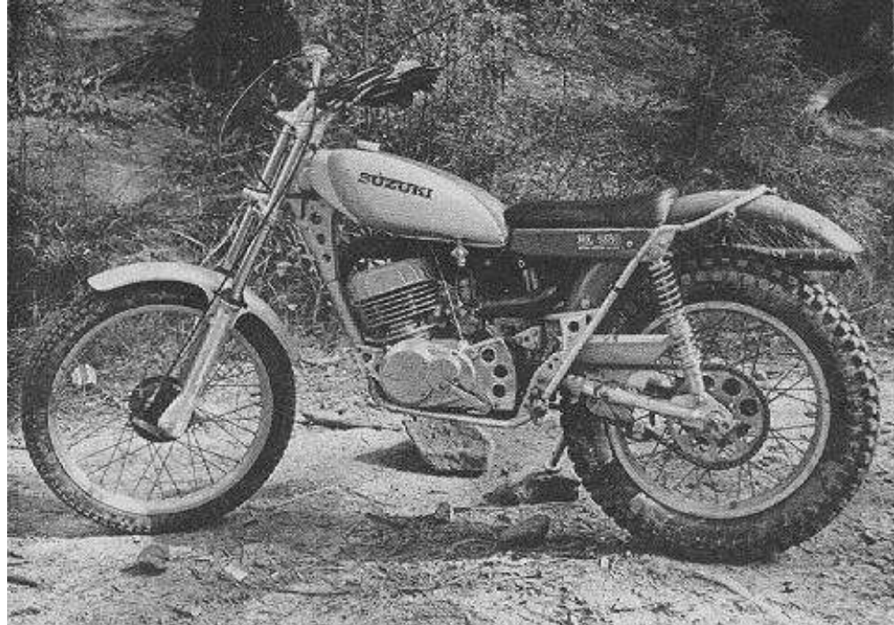
Suzuki's RL250 demands a delicate touch. The light front end means easy up-and-over tactics, but the extremely quick steering can be a drawback when the going gets tight. It's not a bike for the trials novice.
